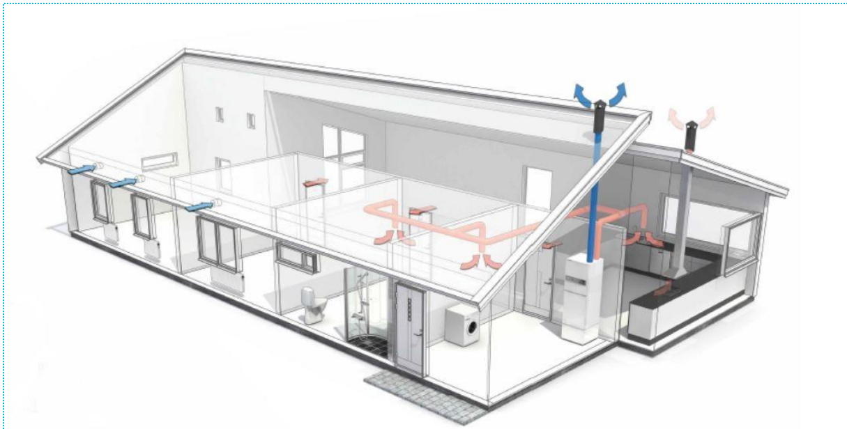
Figure 3 - Exhaust air heat pump flow diagram
