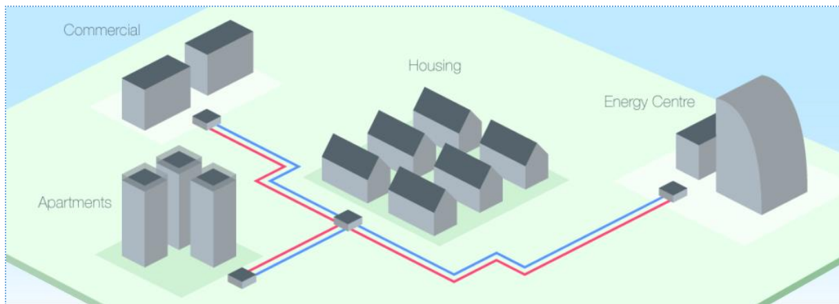
Figure 8- Typical district heating flow diagram
